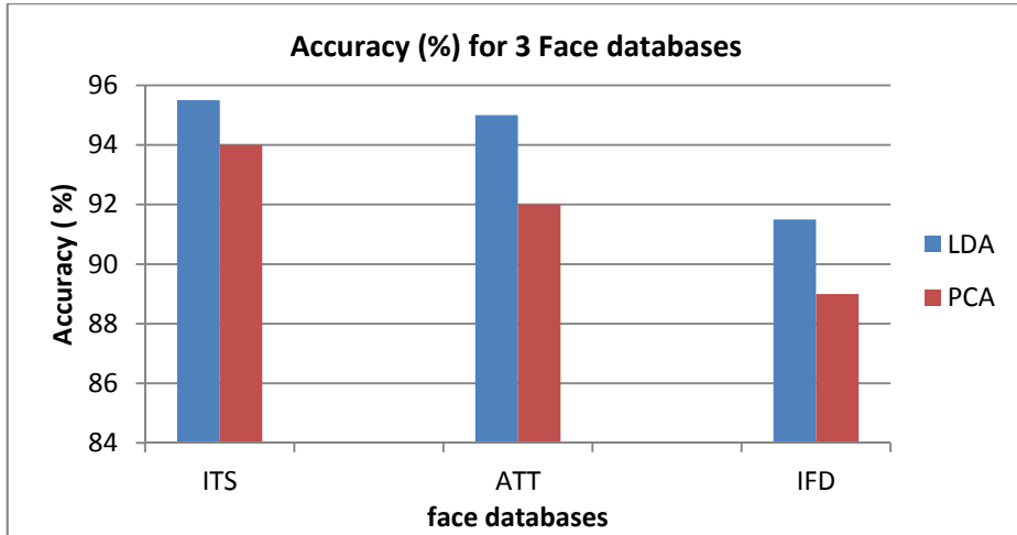
Fig. 4. Success rate comparison of face recognition between 3 faces databases, each using 10 sets face. It shown clearly that ITS database have highest success rate than ATT and Indian face database when the illumination of testing images is varied. The success rate using PCA in our proposed method and ITS face database is 95.5 %, higher than ATT face database 95.4%.
