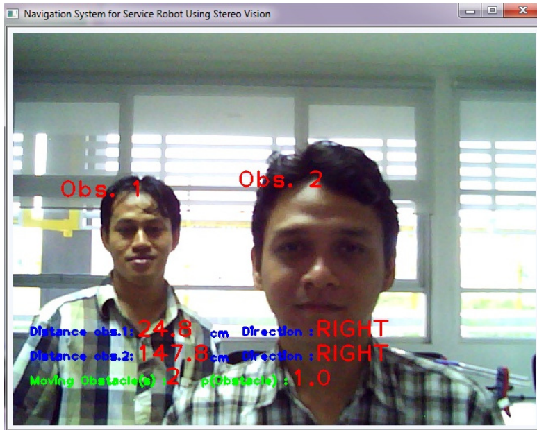
Fig. 8. Robot successfully identified and estimated distance of 2 moving obstacles in front of robot.
